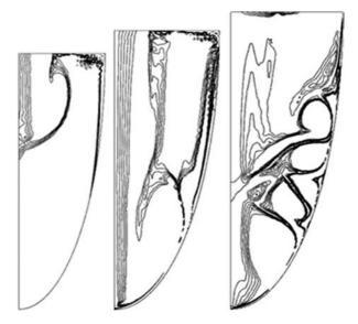
Figure 4. Vortex formation patterns obtained using parabolic velocity profile as inlet boundary condition at t = 0.15 s (left), 0.25 s (middle) and 0.35 s (right).
